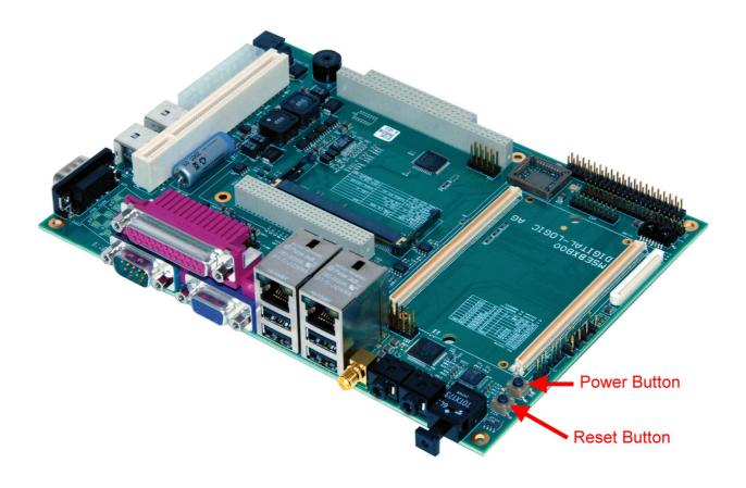
**Power Button:** Push the Power Button for 2 seconds to start up the system.
